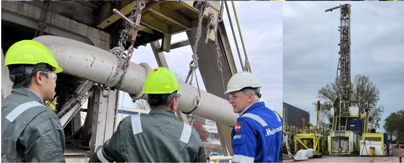
Pictures during onshore drilling visit in Delft, Netherlands on the 9th November 2023. The LOC400 3 rig is a modern, compact rig currently drilling geothermal wells. Visit was joined by representatives from Huisman, Vanguard Drilling, NRG Group and Upland Board and Executives.
